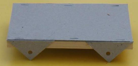
A basic chassis is assembled and ready for the wheels and axles to be added.
