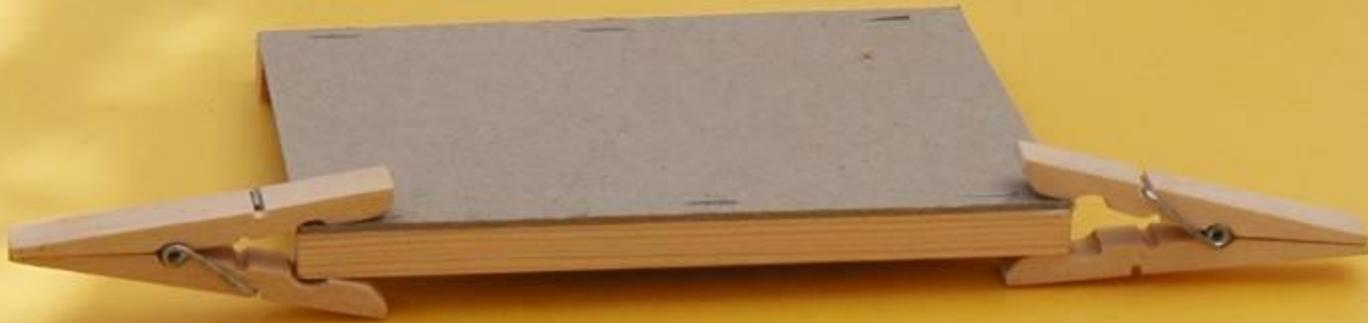
Clothes pegs are used to clamp the card to the wood whilst the PVA glue dries.
