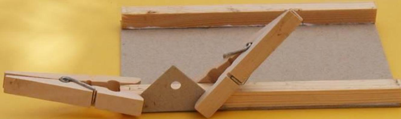
Axle holders (bearings) are positioned and glued in place.
